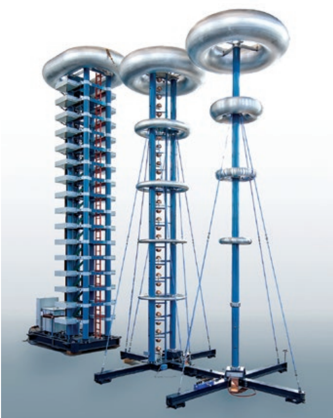
Fig. 1 Impulse voltage test system series G with Connection Point
