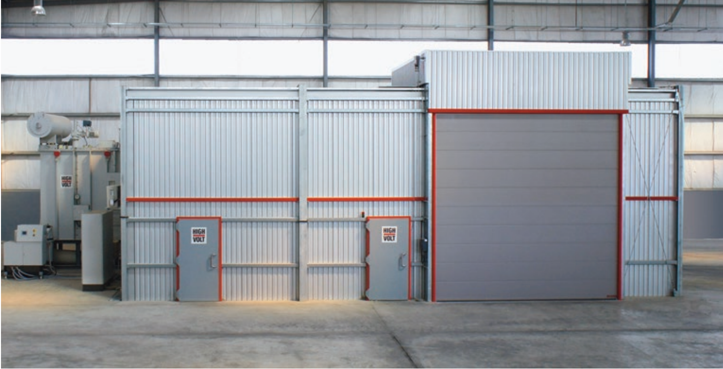
Fig. 1 Shielded room SSC 15x9x5.6 with integrated AC resonant test system WRU 10000/350-200-100 for routine testing of high-voltage cables
