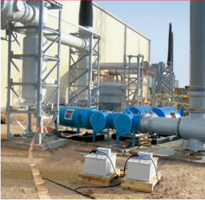
Fig. 1 AC resonant test system type WRVG G for on-site testing of GIS/GIL
