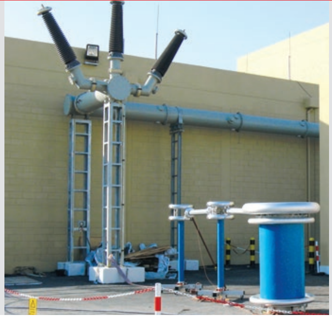
Fig. 2 AC resonant test system type WRV M for on-site testing of GIS/GIL
