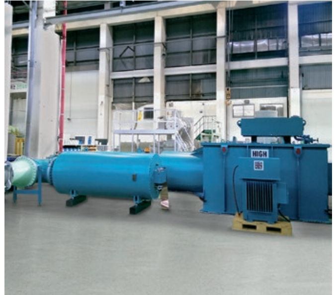
Fig. 10 AC test system WRVG 5.7/750 G (gas-insulated reactors, left side) and WRV 6/750 G (oil-insulated reactor, right side)
