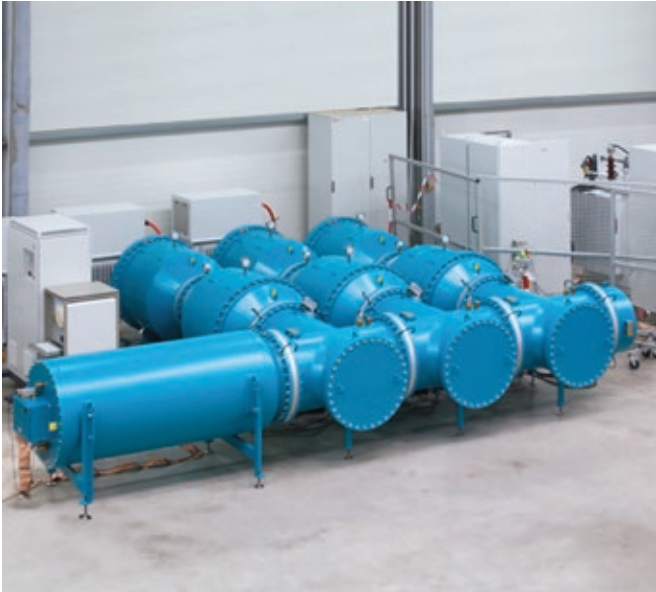
Fig. 10 AC test system WRVG 5.7/750 G (gas-insulated reactors, left side) and WRV 6/750 G (oil-insulated reactor, right side)
