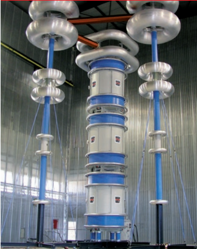
Fig. 1 HVAC resonant test system type WRM
