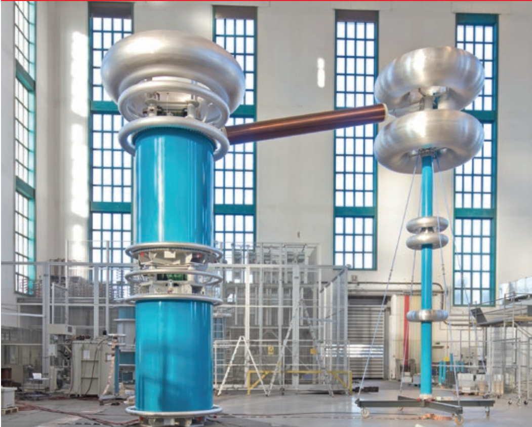
Fig. 1 HVAC cascade based on insulating case transformers type WP 1000/1000
